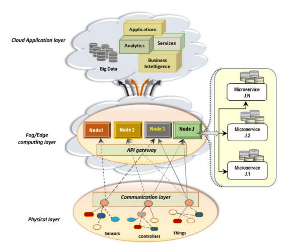
**Figure 2. The four-layered model using Fog/Edge computing level** (Source: designed by the authors considering the Cisco IoT Reference Model)
