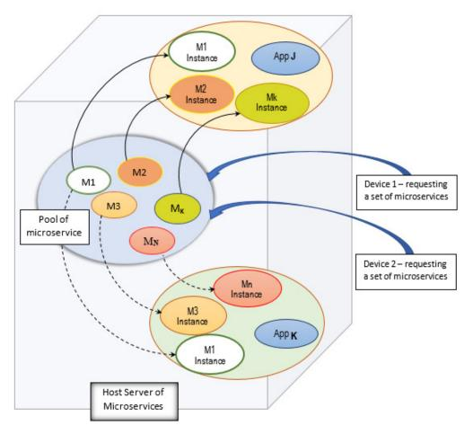
Figure 1. Microservice-based architecture
