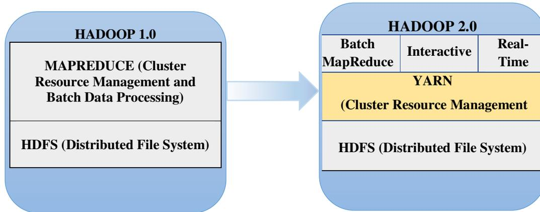
**Figure 2. The architecture diagram of Hadoop 1.0 and Hadoop 2.0/YARN**
