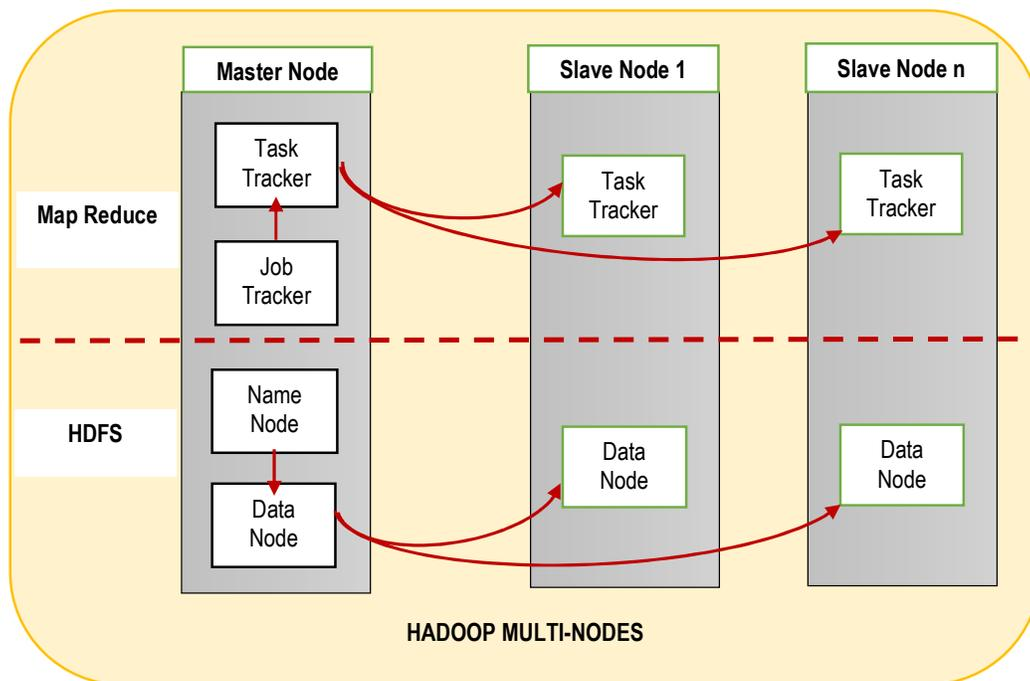
**Figure 1. The structure of a Hadoop cluster** (Source: Gupta, 2014)
