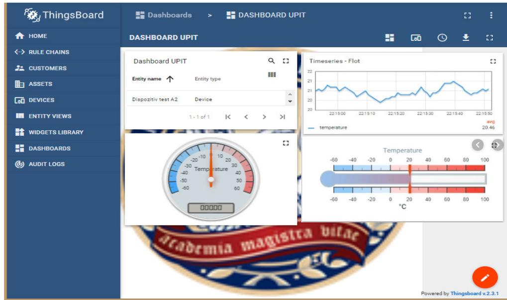
Figure 4. Creating a dashboard for monitoring devices
