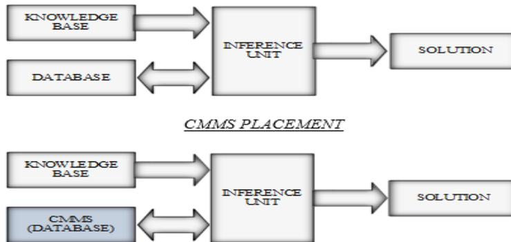
**Figure 3 Structure of expert system and structure with the placement of CMMS**
