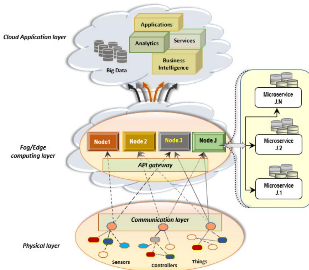
**Figure 2. The four-layered model using Fog/Edge computing level**
