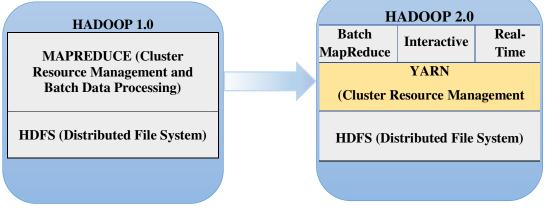
Figure 2. The architecture diagram of Hadoop 1.0 and Hadoop 2.0/YARN Source: http://hortonworks.com/blog/how-to-plan-and-configure-yarn-in-hdp-2-0/
